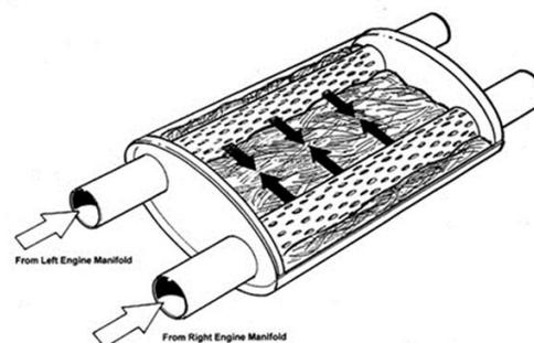
Advantex® fibers can maintain mechanical integrity for temperatures above their continuous operating temperature limit (740°C) for varying periods of time. To determine whether blowout might occur for particular time/temperature operating conditions, it is recommended that direct contact be made with Owens Corning for technical assistance.
